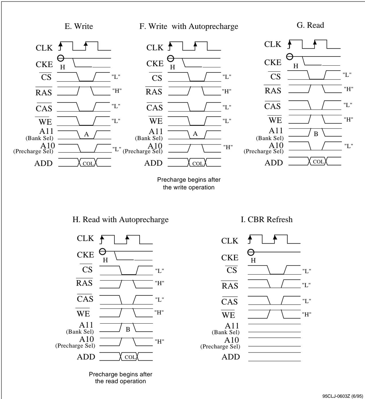
**Figure 3-2. Command Timing Diagrams (3 of 3)**
