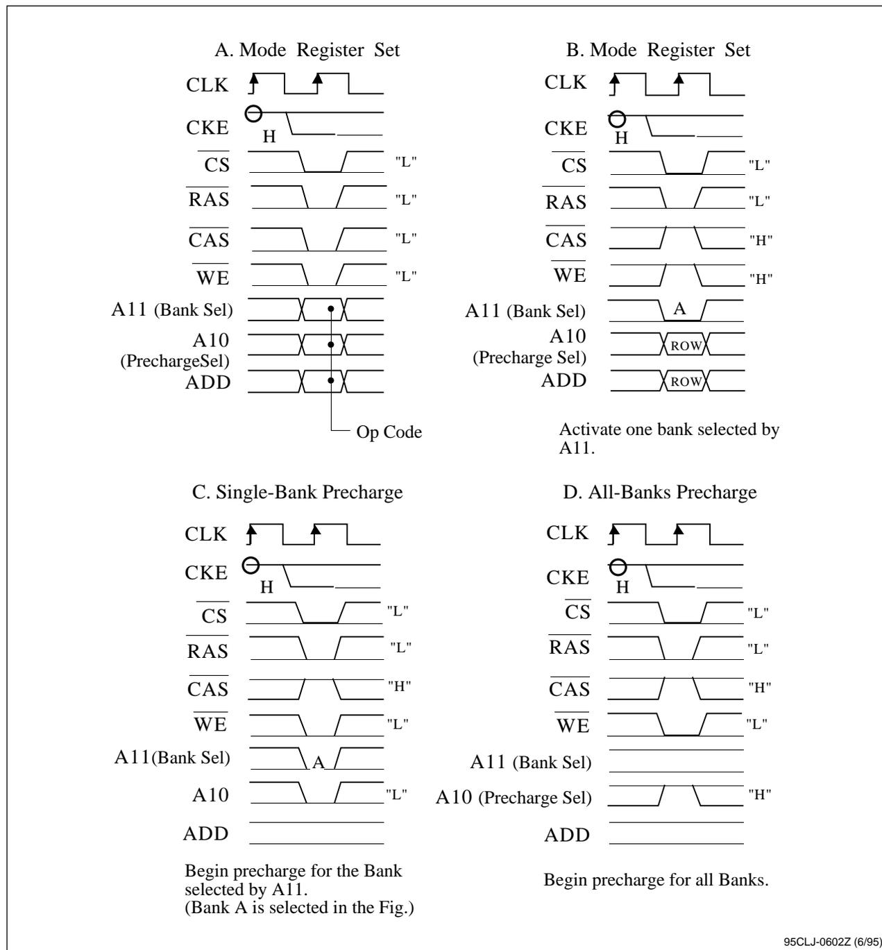
Figure 3-2. Command Timing Diagrams (2 of 3)
