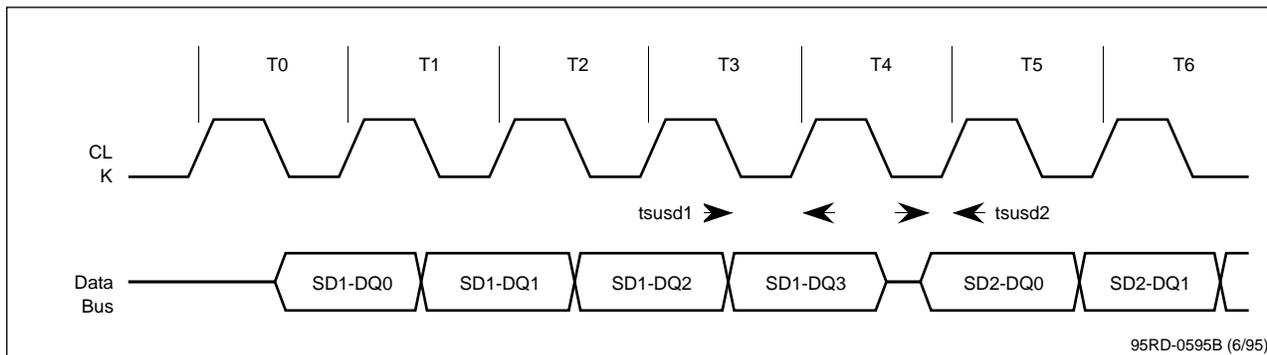
The difference in flight time between SDRAM1 and SDRAM2 to the memory controller is the difference in time Tdelta. Further, the overall clock skew (Tskew) and the memory controller setup (Tsetup) times must be added to the equation. Thus, the following equation is used to derive the the true system timing required to satisfy the available data window for the controller:
