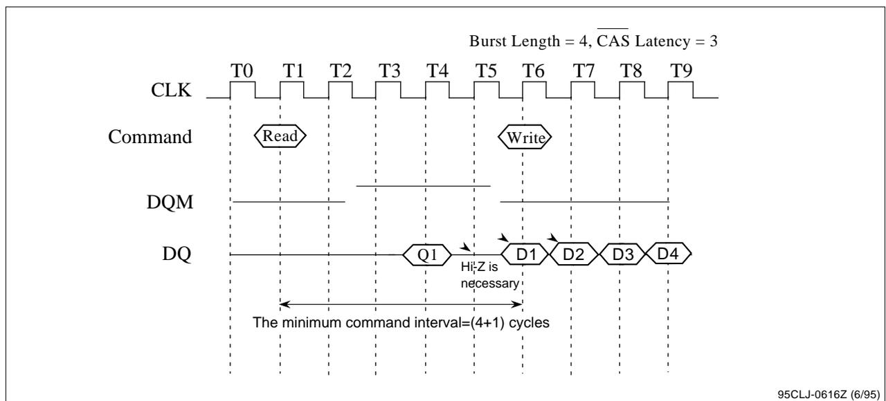
When the  $\overline{\text{CAS}}$  latency = 3 for any burst length except full page, a read can be interrupted by a write but the minimum command interval between Read and Write equals the burst length plus 1. This rule has one exception: a dummy Write command
