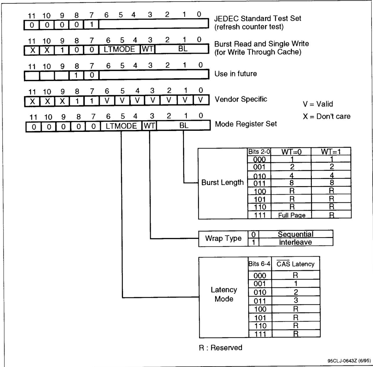
Figure 5-7. Mode Register Set Example
