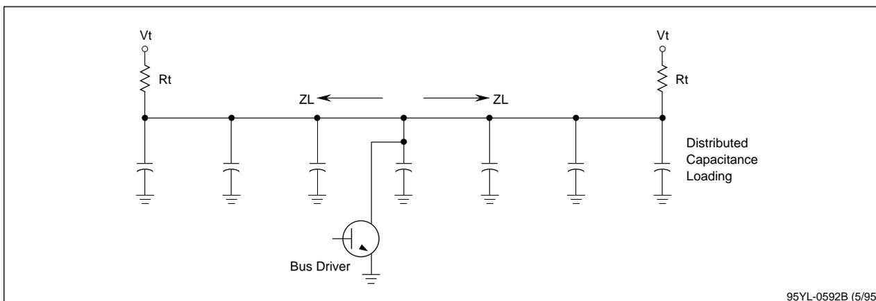
To drive the bus properly requires a driver capable of the following:
