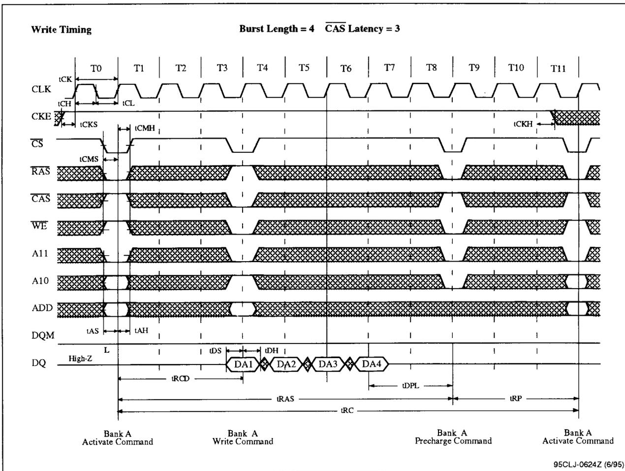
**Figure 4-4. Write With Auto Precharge Timing**
