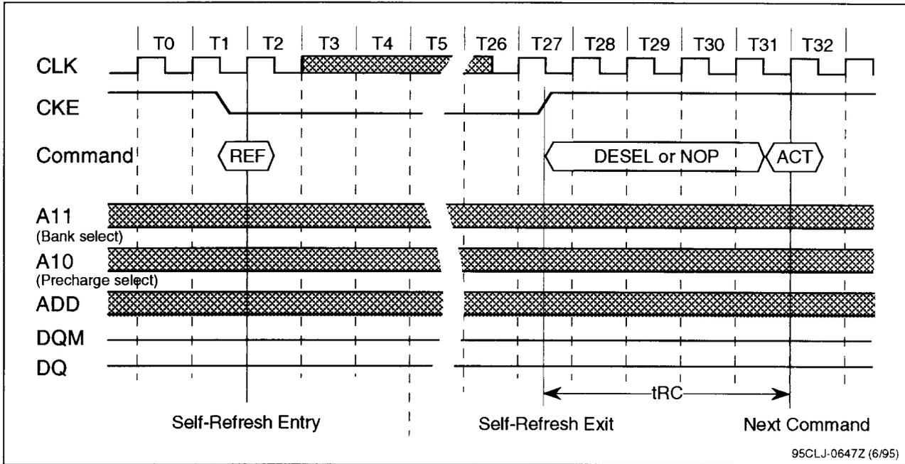
**Figure 5-11. Burst Refresh Timing**
