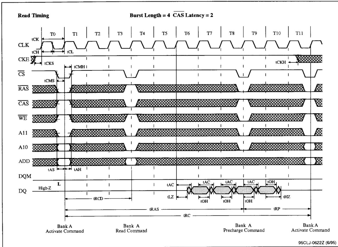
**Figure 4-2. Read with Auto Precharge Timing**
